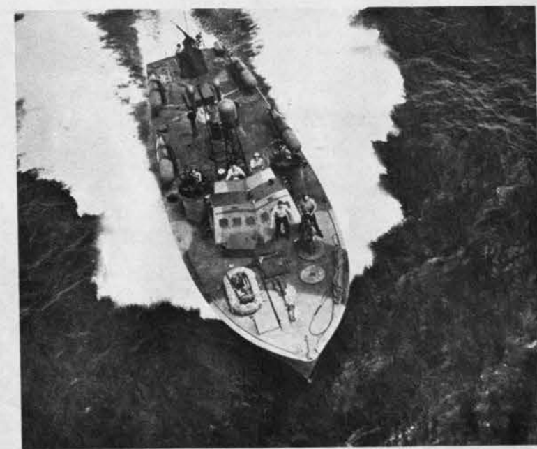
Broad curved deck of U. S. PT carries more cannon and MG's than Japs'. Flaring lines and four torpedo mounts stand out in contrast.
